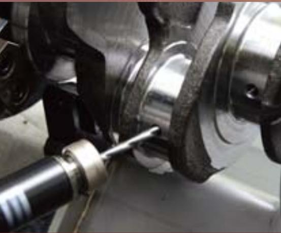
MQL Drilling System for Crankshaft
